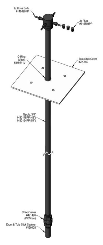
PREVENTIVE MAINTENANCE: When the unit will be out of service for extended periods, place chemical tube(s) in water and flush the chemical out of the unit to help prevent chemical from drying out and causing build-up. Periodically check and clean chemical strainer and replace if missing.
