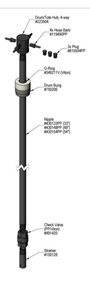
PREVENTIVE MAINTENANCE: When the unit will be out of service for extended periods, place chemical tube(s) in water and flush the chemical out of the unit to help prevent chemical from drying out and causing build-up. Periodically check and clean chemical strainer and replace if missing.
