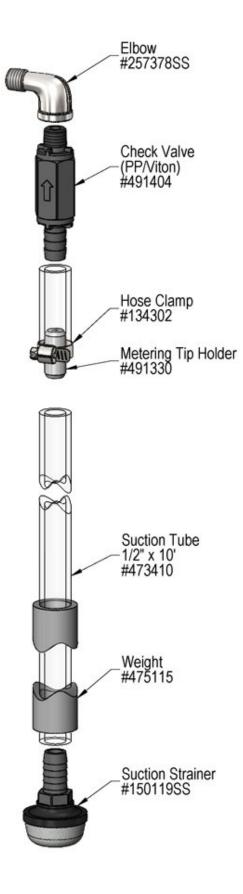
PREVENTIVE MAINTENANCE: When the unit will be out of service for extended periods, place chemical tube(s) in water and flush the chemical out of the unit to help prevent chemical from drying out and causing build-up. Periodically check and clean chemical strainer and replace if missing.
