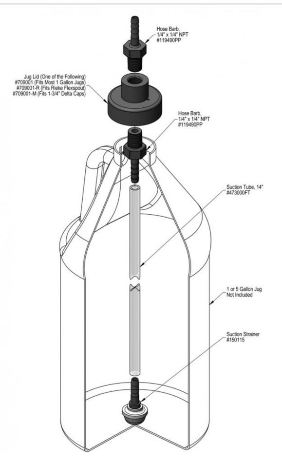
PREVENTIVE MAINTENANCE: When the unit will be out of service for extended periods, place chemical tube(s) in water and flush the chemical out of the unit to help prevent chemical from drying out and causing build-up. Periodically check and clean chemical strainer and replace if missing.
